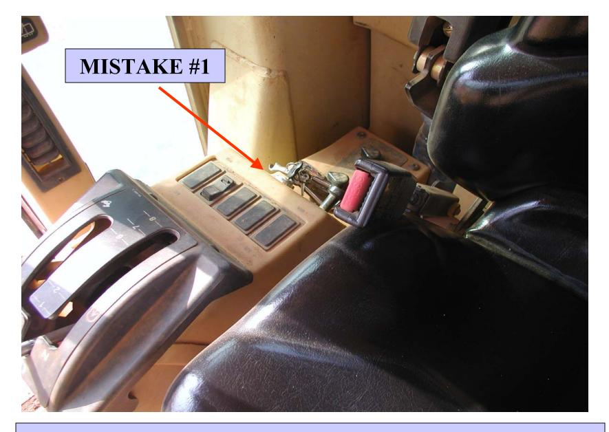
OPERATOR LEFT CAB WITH EQUIPMENT RUNNING
