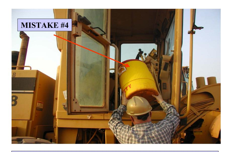
OPERATOR LOADS MATERIAL INTO GRADER CAB
