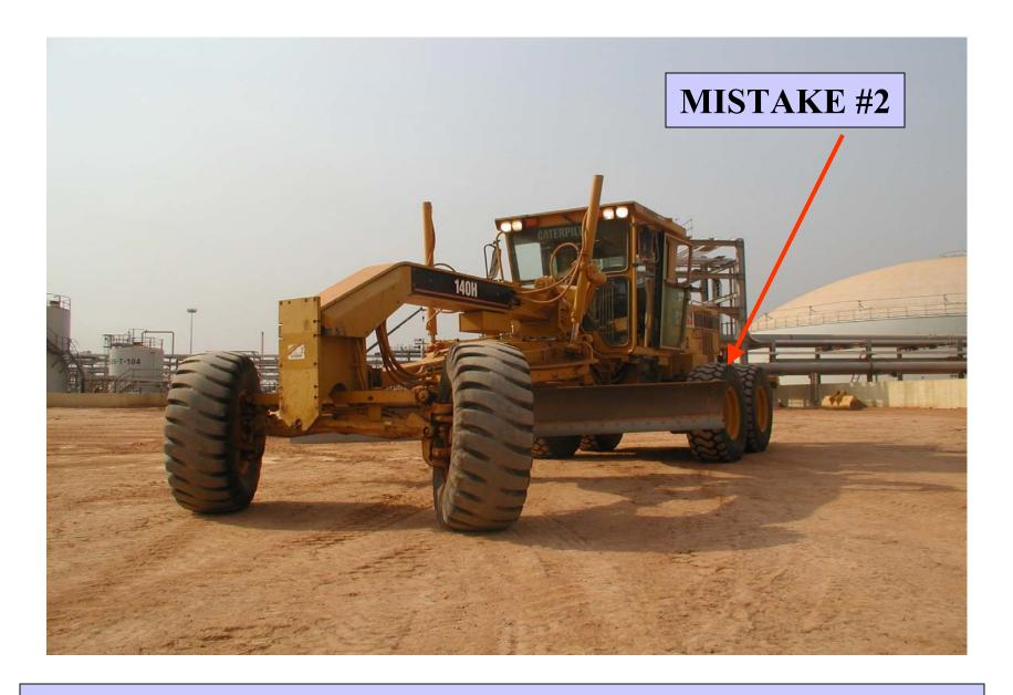
OPERATOR LEFT CAB WITH BLADE AND RIPPER UP.
