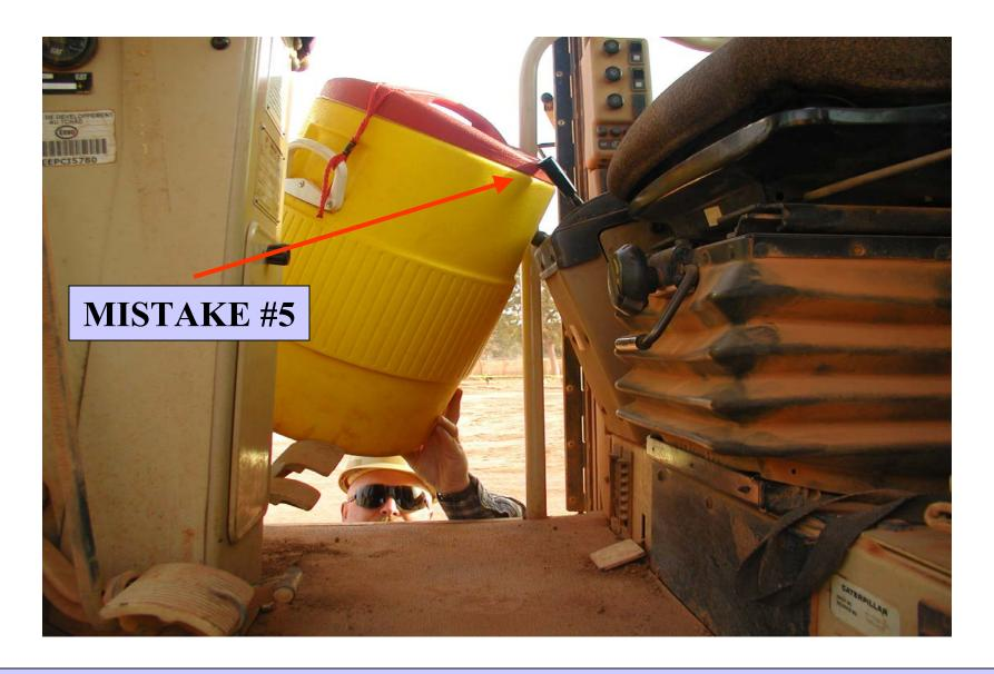
OPERATOR HITS GEARSHIFT AND PLACES EQUIPMENT INTO 1ST GEAR
