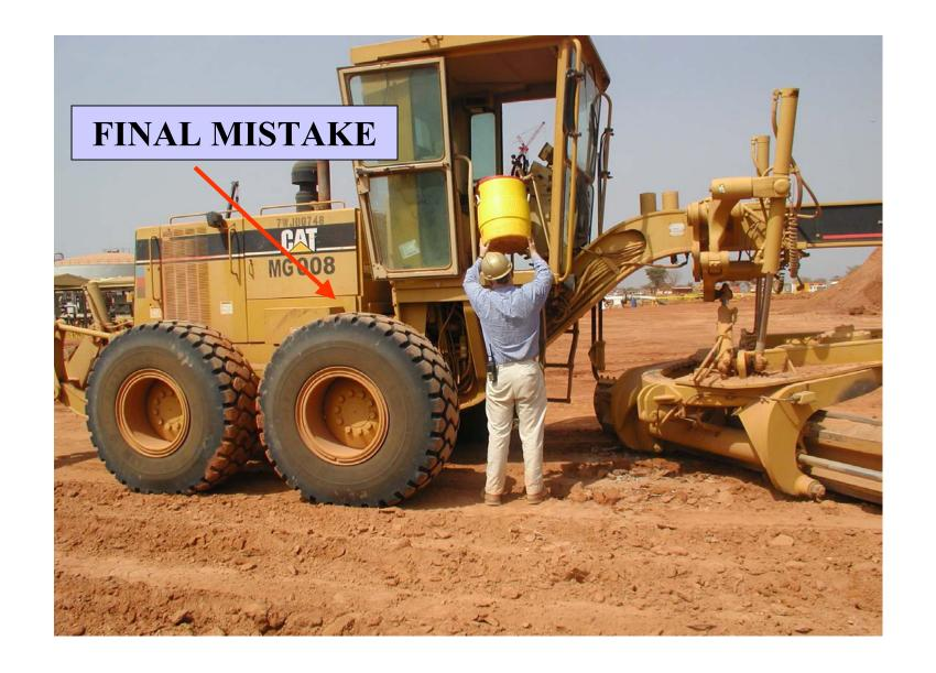
OPERATOR CRUSHED WHEN EQUIPMENT MOVES FORWARD
